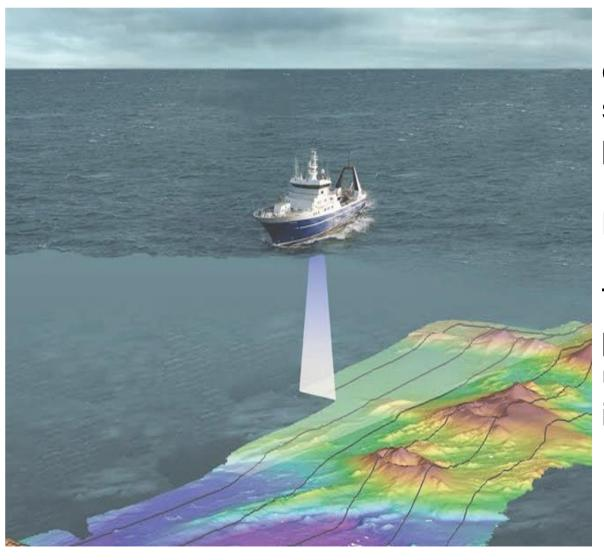
Using subsea scanning sonar equipment and positioning to detect seabed surface debris and possible prior spud-can penetration sites can reduce the risk of damage to Jack-up MODU legs.
