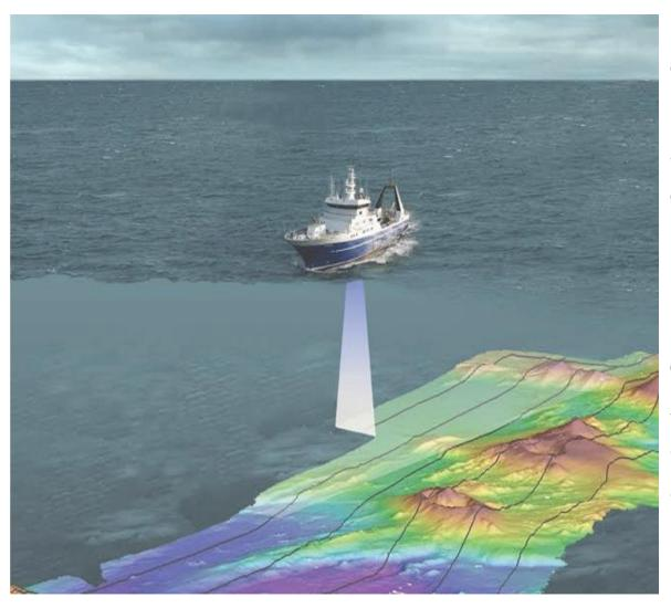
Creating detailed bathymetric charts of drilling and construction locations is essential for the design of infrastructure and the carrying out of offshore operations.
